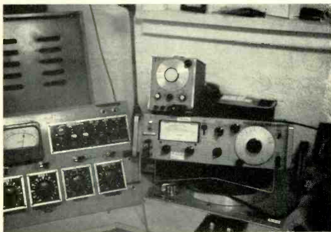
Fig. 2. Hewlett-Packard 334A Distortion Analyzer and 204D Oscillator in use at KLOY-AM-FM, Loveland.
