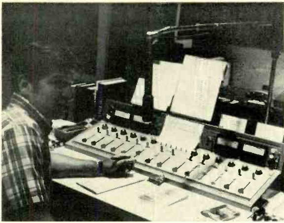
Announcer Marty Robinson prepares for a newscast at console which has dual stereo output channels and four VU meters.
